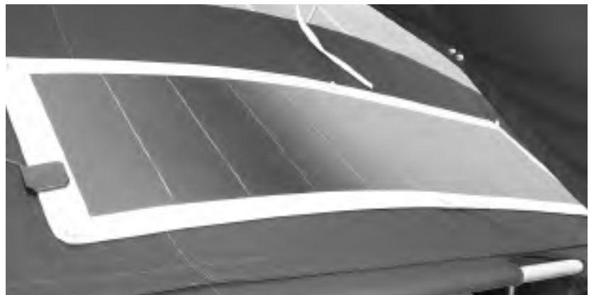
Uni-Solar FLX 32 mounted on dodger
