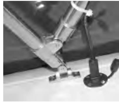
Location of waterproof connector for solar panel
